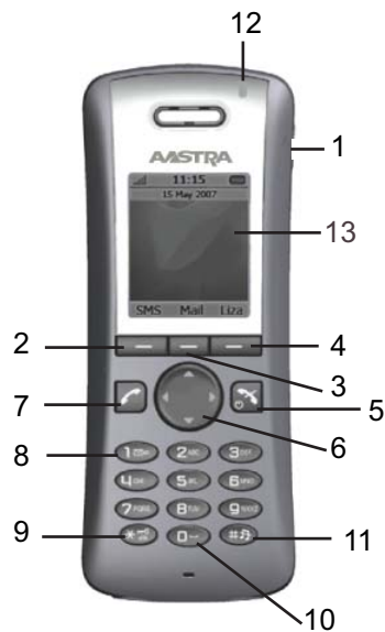
Figure 1 Overview of the cordless telephone DT390
